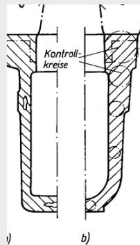
a) Cavity due to unfeedable material accumulation
