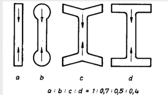
The examples above illustrate the different shrinkage restraints in the direction of the arrow for different geometries, showing the relative shrinkage ratios. The internal stress in the component increases with increasing shrinkage restraints.
