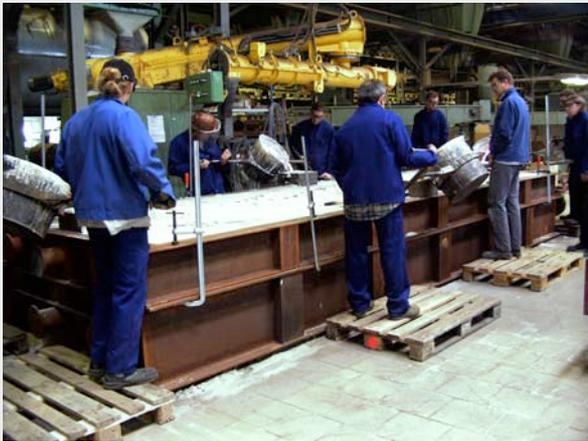
New guidelines and laws for ecological production and environment protection confirm now - although rather late - that we did it right, as the Sodium silicate method belongs to the non-organic and odourless foundry binders. When burning the binder neither formaldehyde nor phenol will be set free as it would with organic binders. Hence, the impact on employees, neighbours and the environment is very low - during molding as well as during disposal.
