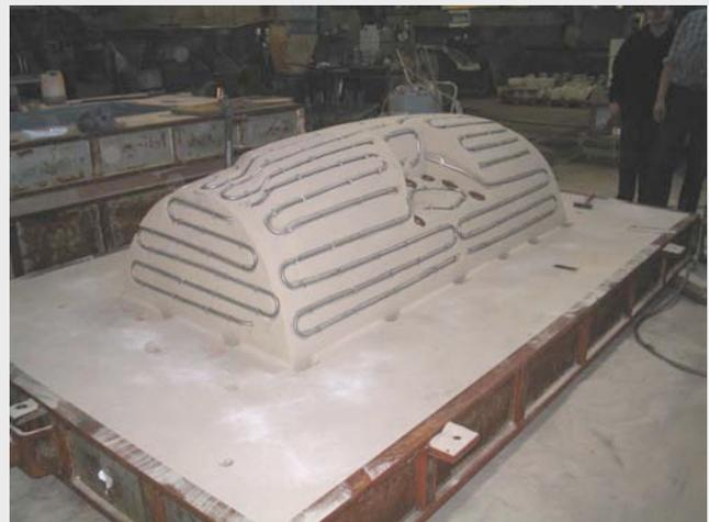
As molding material we use green sand, just like in the rest of our molding lines. However, when we have to cope with very complex, heavy, narrowly tolerated, very challenging or big geometries, the consistency of green sand is not sufficient. In order to serve these customer requirements as well, we produce the molds with the 'Sodium silicate - Ester' method. Sodium silicate consists of an alkali silicate (Na, K, Li), silicium (oxygen acid of silica) and water solution.
