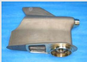
For our customer Volvo Penta we have enhanced the approved sea water-resistant alloy G-CuAl10Ni to be able to produce environmentally friendly oil-proof cast parts with demanding inner contour. It is used in components of the innovative IPS-Drive of Volvo Penta that are completely hanging in the sea water. These two cast parts are weighing 61 and 63 kg, and by using a special heat treatment they stay resistant to corrosive attacks.
