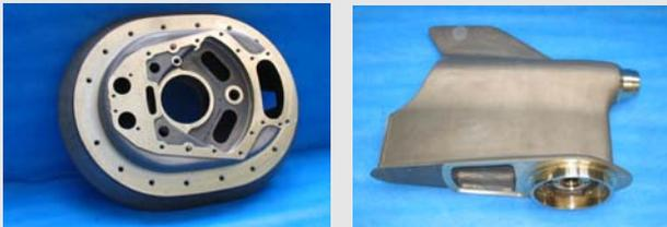
For our customer Volvo Penta we have enhanced the approved sea water-resistant alloy G-CuAl10Ni to be able to produce environmentally friendly oil-proof cast parts with demanding inner contour. It is used in components of the innovative IPS-Drive of Volvo Penta that are completely hanging in the sea water. These two cast parts are weighing 61 and 63 kg, and by using a special heat treatment they stay resistant to corrosive attacks.
