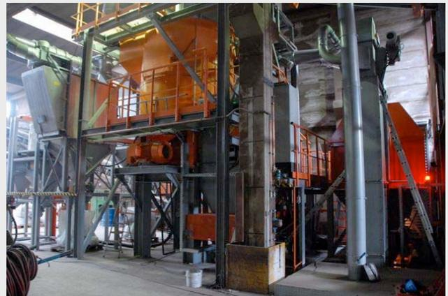
Afterwards the sand is transported into the heart of the plant: the mixer. But before this, it is weighed and its consistency, e.g. temperature and water content, is measured. This information is included in the calculation of the recipe. The sand recipe of each batch is different: the staff of each molding line sets the sand quality they need for the current production, which is different from line to line and from one pattern to the other.
